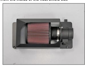
9. Install the K&N® air filter onto the mass air sensor inside the heat shield and secure with the provided hose clamp.
