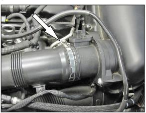
3. Loosen the hose clamp which secures the intake tube to the mass air sensor.
