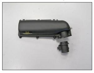
6. Remove the two screws securing the mass air sensor to the upper air box housing and then remove the sensor as shown.
