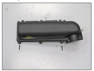
11. Remove two of the upper air box mounting bolts as shown.
