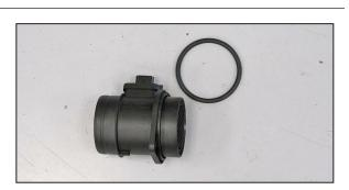
7. Remove the factory O ring from the mass air sensor.
