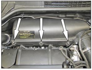
4. Loosen the three screws securing the upper air box housing to the lower housing.
