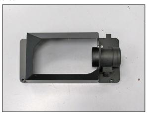
8. Install the mass air sensor into the  $K\&N^{\otimes}$  heat shield using the provided hardware.
