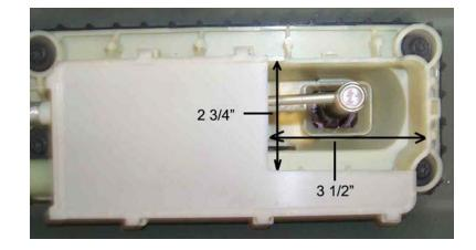
9. Cut the dust cover as indicated for clearance of the new shifter extension
