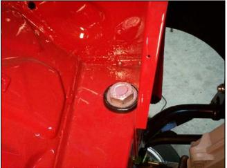
Step 3: Drill six holes to support the bottom of the subframe using a 5/16" drill bit. Use the six supplied 5/16" bolts with plates to fasten the subframe to the car on the lower side. The plates will go inside of the car to give the floor panel extra support. After the six bolts are in place and tightened, tighten the two large subframe mounting bolts on top of the frame. See photos.
