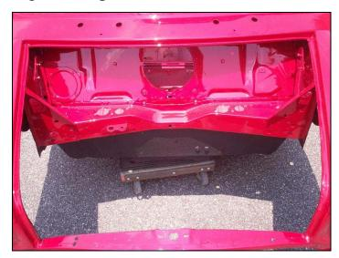
**Step 2:** Whether you use Mini Tec's MT Flip Front End Kit or you do an extension yourself, you will need to cut existing Mini front end after the a-panel seem to remove existing Mini front. See Figure 1-2. Note: For extended metal front ends, it is best to attach the MTK subframe first before performing any body extensions.
