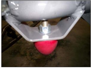
**Step 2:** Attach the subframe to the car using the two large subframe mounting bolts just like the standard Mini subframe. If your car is an earlier model and does not have these two large ¾" diameter bolts, then you will need Mini Tec's MK1/2 Subframe Mounting Kit (#351000). Standard Mini mounting bolts are circled in red in the following photo. Do not tighten completely at this point. You will need to attach the subframe and the bottom first.
