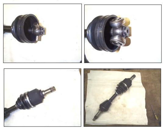
**Axle Installation:** Simply slide one of the axles into the transmission and the other into the engine mid-shaft until the axles lock into place.
