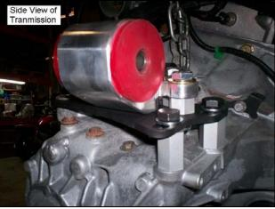
**Step 3:** Attach Honda B Series engine mount (#210280) to MTK frame as shown. Make sure that your mount is for a Honda DC chassis.
