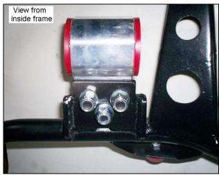
**Step 4:** Attach MTK engine mounting bracket to engine block as shown. For some engines, you will need to use the supplied spacer plates for clearance.
