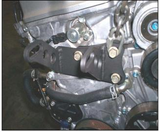
Step 5: Lower engine into subframe and attach it with the hardware provided.
