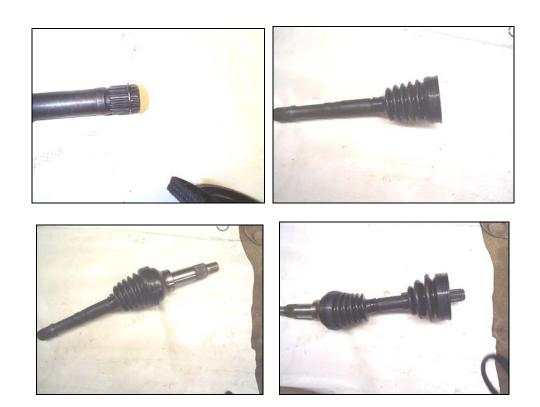
**Honda Axle End Assembly:** Assemble large splinned side of axle with the Honda cv joint assembly. (See following four Photos)
