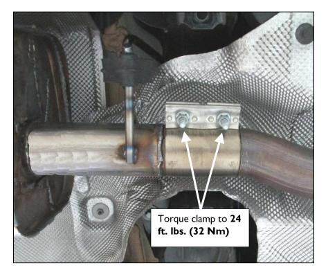
8. Install sub-frame brace using the 2 bolts you saved from disassembly.
