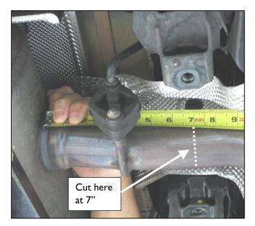
3. Remove stock muffler from rubber hangers as shown in **Figures 3 and 4**. Using spray lubricant on the muffler hangers will help with removal.
