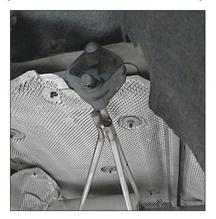
7. With exhaust clamp rotated as shown, torque clamp to 24 ft. lbs. (32 Nm).
