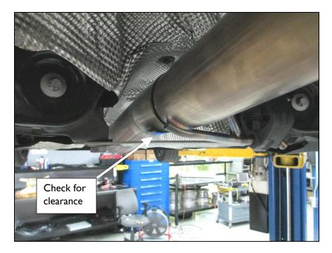
10. Be sure to check for proper clearance between the exhaust tips and bumper.
