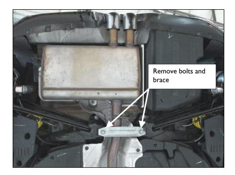
2. Support the muffler securely with a jack or a stand, then cut the stock muffler 7" away from the front of the stock muffler as shown in figures below. Before cutting the stock muffler, hold DINAN muffler underneath stock muffler to verify the stock pipe will not be cut too short!
