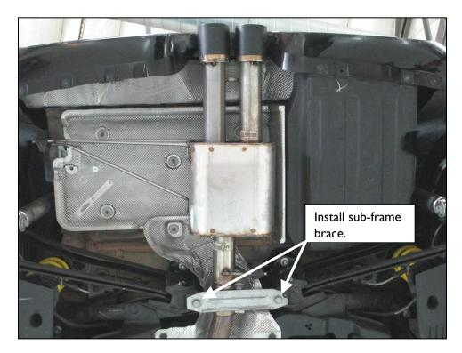
9. With muffler fully installed, be sure to check for proper clearance between the exhaust pipe and sub-frame brace.
